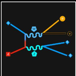
Quarks from the collided nuclei can interact to emit bosons, one of which decays to more quarks, and the other to a muon and a muon neutrino. In the detector, the quarks form jets in the calorimeters. Muons are picked up as hits in the muon spectrometer. The neutrino flies straight through the detector: we infer it was there by the amount of missing energy!
